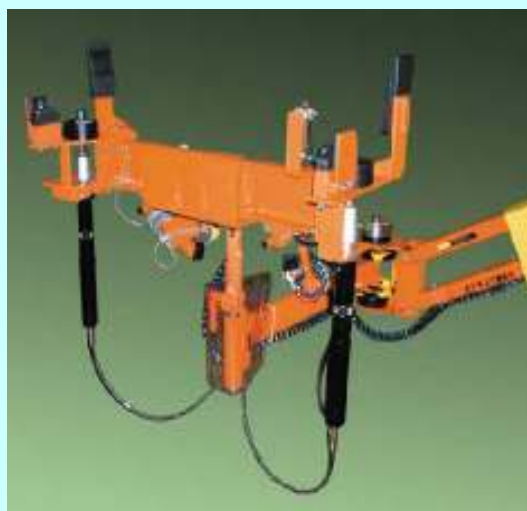
下部締め付け(位置決め付) Tighten from under the vehicle with positioner
