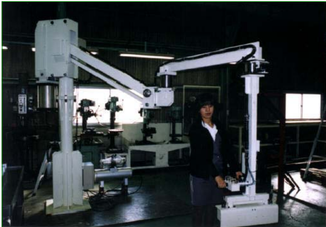
Type 200 Transfer of metallic molds
